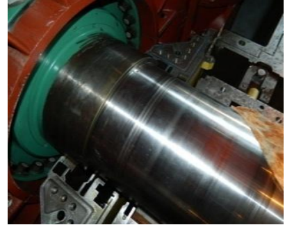
GENERATOR ROTOR SHAFT 500 MM DIA.
