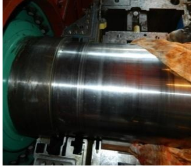
GENERATOR ROTOR SHAFT 500 MM DIA.
